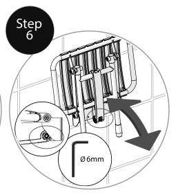
Check the seat operation, levels and leg positioning when it is raised and lowered. To adjust the rate the seat lowers, tighten the linkage bolt under the seat with a 6mm Allen key.
