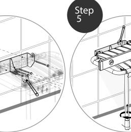
Do-not over-tighten fixings and do not use countersunk screws as these can reduce the strength of the seat and will invalidate any warranty or weight capacity stated.
