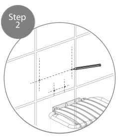
Identify the most appropriate position for the shower seat ensuring the product is at a comfortable height and distance for showering. The product can be folded upwards for more convenient storage so please ensure there is sufficient space above the fixing to allow for this.
