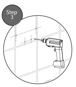
Drill the holes to a depth suitable for the wall fixings you have chosen. Do not drill through the tiles using a 'hammer action' on the drill as this can crack the tiles.
