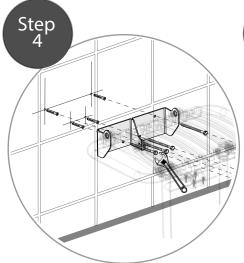
Use suitable wall fixings to secure the mounting bracket to the wall.
